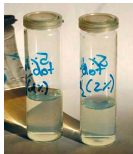
Figure 2: 10 % by weight particle suspensions of Na-doped particles with 1 % and 2 % sodium.
