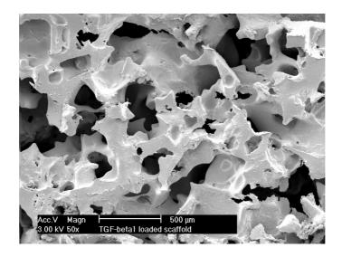
Fig. 1 Cross sections of a TGF- $\beta$ 1-loaded porous scaffold examined by scanning electron microscopy.
