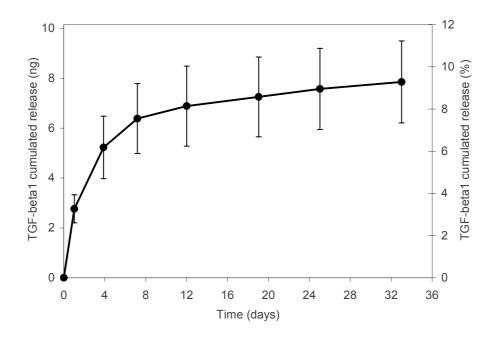
Fig. 2 Cumulated release of TGF- $\beta$ 1 from 4×4 mm cylindrical porous polymeric scaffolds. At each time point, the release medium was collected and the amount of growth factor released quantified by ELISA. (n = 3 ± S.D.).
