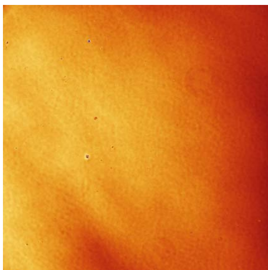
a) (\text{CeO}_2)_{0.81}(\text{TiO}_2)_1 layer in the EC device with wet electrolyte (after 52000 CA cycles).
