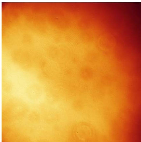
c) \text{WO}_3 layer in the EC device with wet electrolyte (after 52000 CA cycles).
