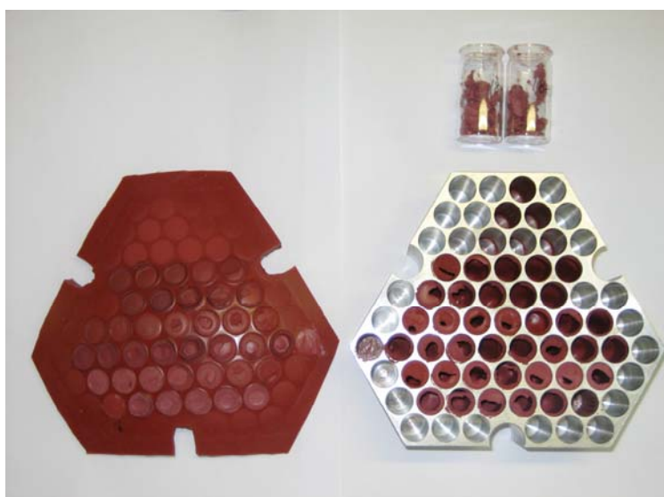
Fig. 4.5 Ex-situ mixed products of the layered pieces in the self-made aluminium rack. Left image is the silicone rubber cover for the rack. Inside the well of the rack is the cooled mixture for different compositions (right-down image). Two of them were taken out and transferred into a glass bottles in order to show the status of the mixture (right-up image).
