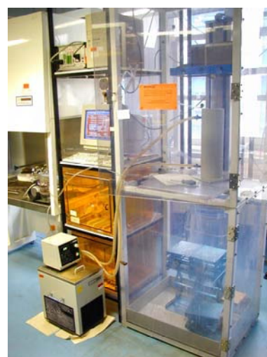
Fig. 1: Dip coating equipment for the inside coating of glass tubes.
