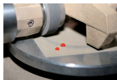
Fig. 3: Taber abraser test – even after 1000 cycles taber abraser test no wetting by water (contact angle against water higher than 90°)
