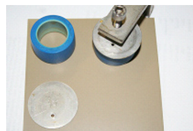
Fig. 3: Experimental setup for determination of chemical resistance of coatings. Blue pot is filled with corresponding test liquid and fixed on the coated substrate.
