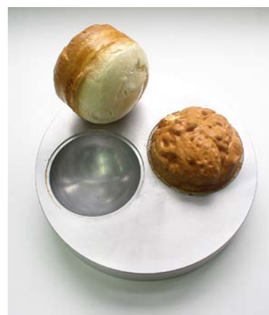
Fig. 4: PU-foam in an aluminium mould, left side with an durable Nanomer® mould release coating
