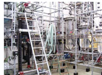
Fig. 1: Process controlled reactors for sol-gel lacquers synthesis
