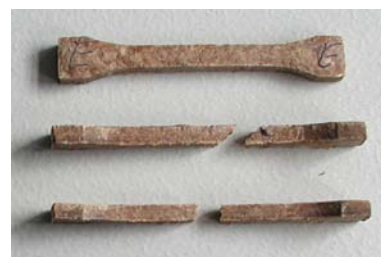
Fig. 3: Tension rods (cellulose-siloxane compound) before/after mechanical test
