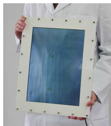
Fig. 8: Curved blue colored EC window of the INM (size 400 mm x 300 mm, curve radius 2000 mm). The transmission in the visible range (TL value, DIN EN 410) can be varied from 70 % (bleached) to 25 % (blue colored, voltage < 3 V, switching time 2-3 min).
