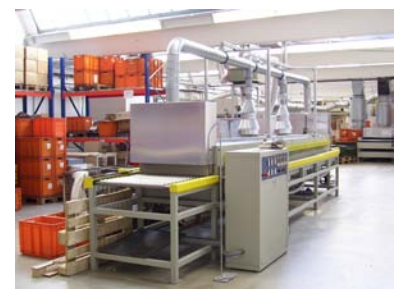
Fig. 2: NMO roller passage kiln for temperatures up to 600 °C
