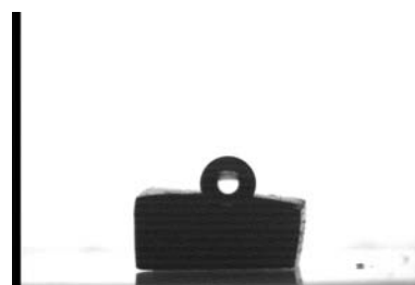
Fig. 1: Coated dental enamel sample, the water droplet demonstrates the low energy surface.
