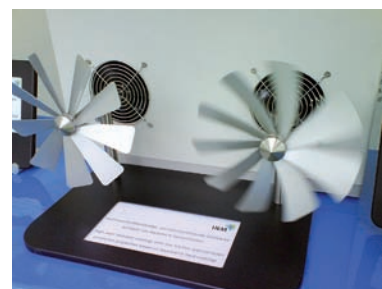
Fig. 5: Windmill with an Nanomer ® coated (right side) and an uncoated (left side) transmission shaft
