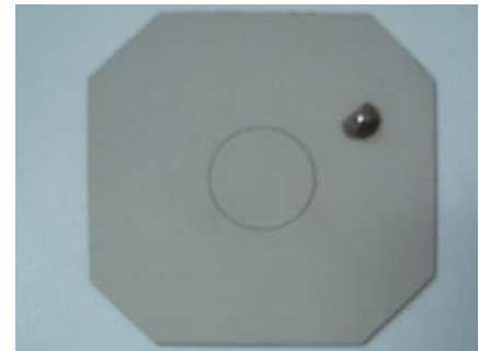
Figure 12: Ball-disc tribometer of glass-ceramic coating (thickness 5 µm) on steel plate (10 cm x 10 cm) after 20 m with 2 N load on stainless steel ball (100Cr6).
