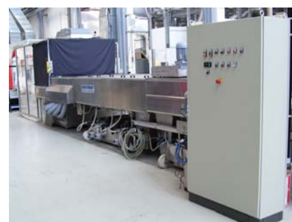
Figure 3: Three step glass cleaning automat (Buxtrup)
