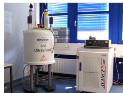
Figure 4: Bruker NMR-spectrometer Avance II with a resonance frequency for protons of 300 MHz.
