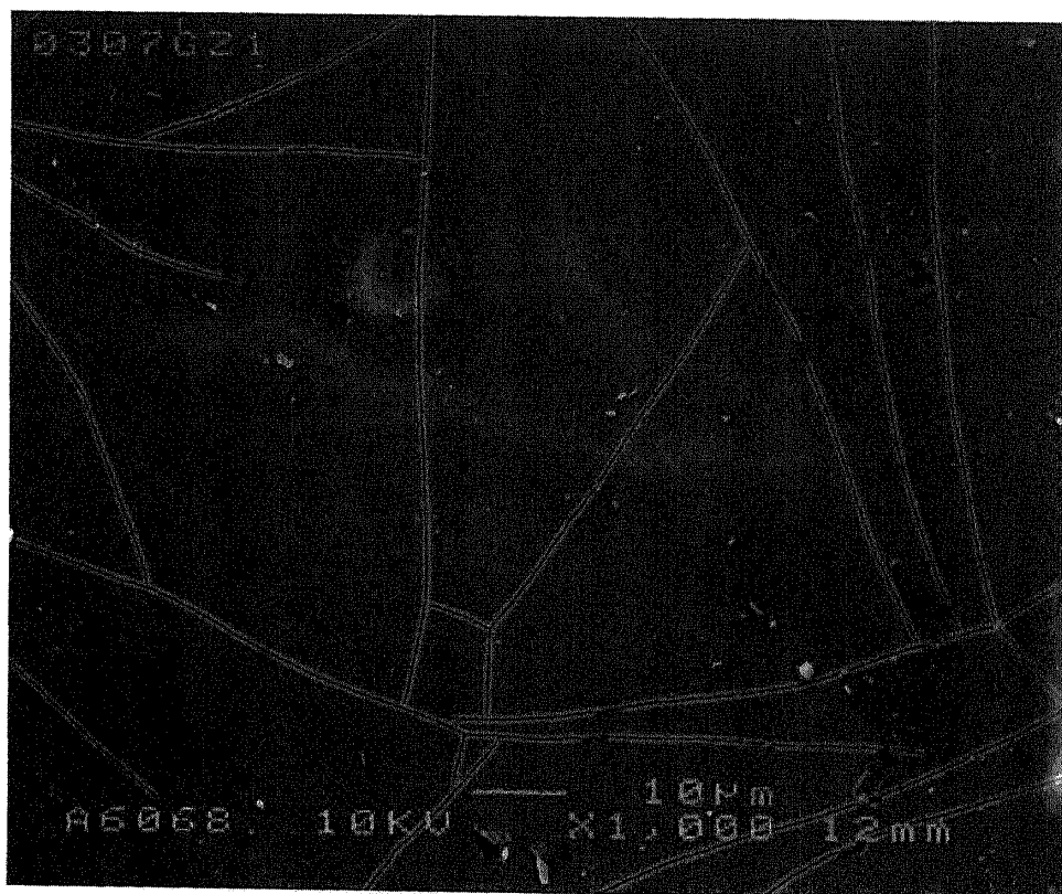
Figure 8. SEM micrograph of the surface of a \text{SnO}_2 : \text{Sb} coating sintered at 700^\circ\text{C} , I = 9 \text{ W/mm}^2 .
