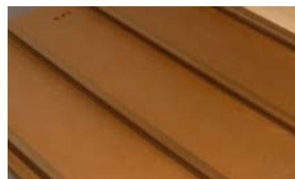
Figure 1: INM-anticorrosion coating on a Multiprotect demonstrator: aircraft skin with welded stringers provided by EADS.
