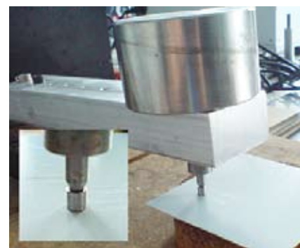
Figure 3: Pin-on-disc abrasion test for linear back-and-forth-movement of the testing head.
