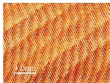
Figure 1: Map of lateral forces recorded on a perfectly flat gold surface in ultra-high vacuum. The atomic structure of the gold surface is revealed through the atomic stick-slip mechanism. Furthermore, the so-called herring-bone reconstruction of the surface modulates the friction force in parallel stripes.
