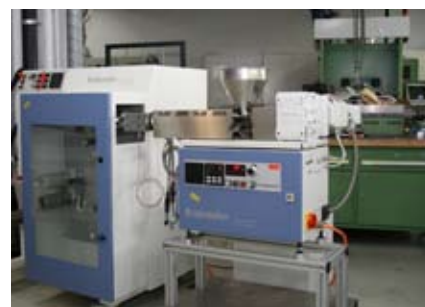
Figure 6: New foil extruder for thermoplastic foil production at the lab scale.
