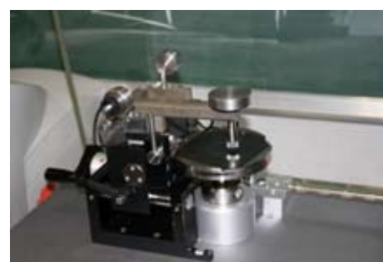
Figure 1: Pin-on-disc tribometer test on Nanomer coated steel plate.
