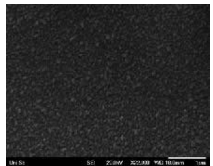
Figure 4: SEM image of the transparent ITO coating.
