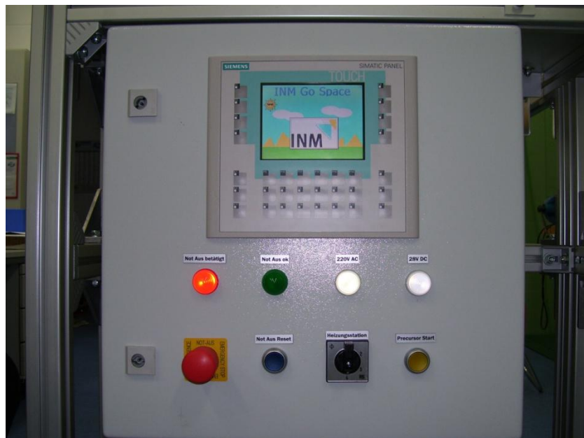
Figure 3-5. Control box of CVD apparatus.
