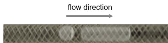
**Figure 4.31:** Zoom on air bubbles flowing from left to right inside the fabric-reinforced tube.
