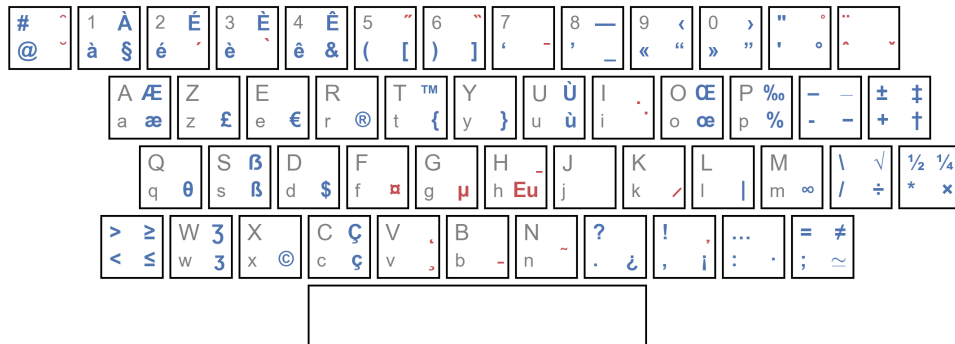
Figure 3.4: The new AZERTY layout [59]. The characters included in the design problem are in boldface and color. Marked in red are dead keys.
