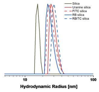
Fig. 1 DLS characterization of the fluorescent particles and pure silica
