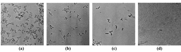
Fig. 11 TEM images of particle removal process. a Particle dispersion before leaching b Removal of particles after centrifugation c Removal of most particles after centrifugation and filtration d filtrate after separation with  $10\,k\text{Da}$  membrane
