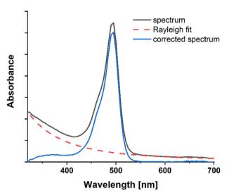
Fig. 12 Example for baseline correction of a scattering sample
