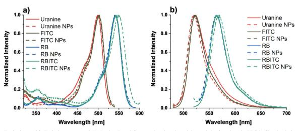
Fig. 3 a Excitation and b Emission spectra of rhodamine B and fluoresceine doped particles and the free dyes in PBS buffered solution
