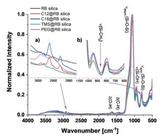
**Fig. 9** . FT-IR spectra of rhodamine B silica NPs and different alkyl functionalized rhodamine B NPs; **a** shows alkyl modes of C12 and C18 functionalized silica, **b** TMS functionalization can be seen via the Si-CH $_3$  mode at 848 cm $^{-1}$
