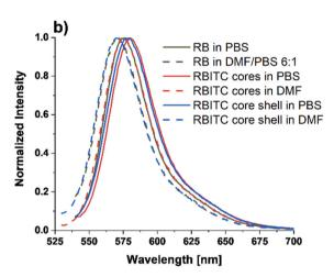
Fig. 4 Spectroscopic characterization of free rhodamine B (RB) and uranine, the core- and core-shell particles in PBS buffer (pH = 7.4) and DMF. a Fluorescence emission spectra of free uranine and
