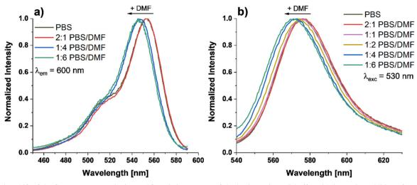
Fig. 5 Blue shift of the fluorescence a excitation and b emission spectra of rhodamine B in PBS buffer with increasing addition of DMF
