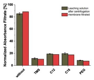
**Fig. 15** Absorbance of leaching filtrates of particles with esterified rhodamine B after 24 h. Leaching behavior of unfunctionalized RB particles with esterified dye is slightly better than without ester bond; an alkyl or PEG functionalization improves the dye retention
