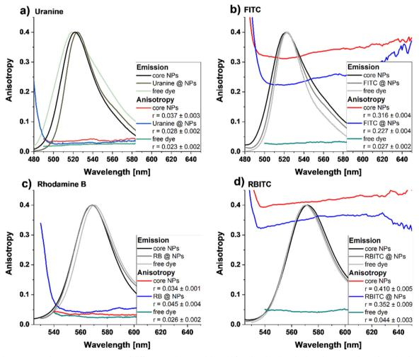
Fig. 6 Fluorescence anisotropy measurements of different xanthene particles and free dyes in ethanol. The anisotropy values of covalently attached dyes are clearly higher than those of the physically attached dyes
