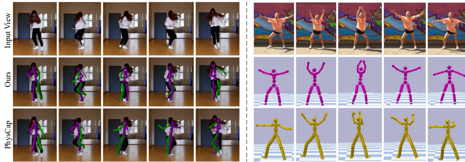
Figure 4.6: Qualitative comparisons of methods with physics-based constraints on videos with fast motions. While having a consistently improved accuracy on general motions compared to PhysCap, our approach can capture significantly faster motions as it learns motion priors and the associated gains of the neural PD controller from data.
