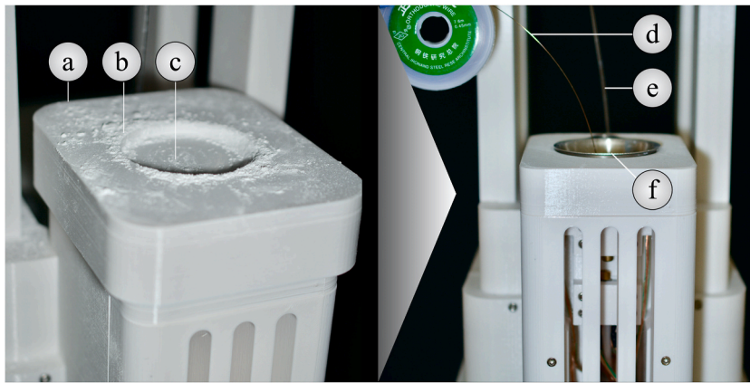
Fig. 6. Cleaning of the coating machine for filament (a) sieve bracket made of Prusament PETG signal white (b) laterally distributed powder of nHA (c) sieve insert made of ColorFabb_HT clear (d) orthodontic wire (e) ColorFabb_HT clear (f) stainless steel funnel for previously added nHA in funnel housing.
