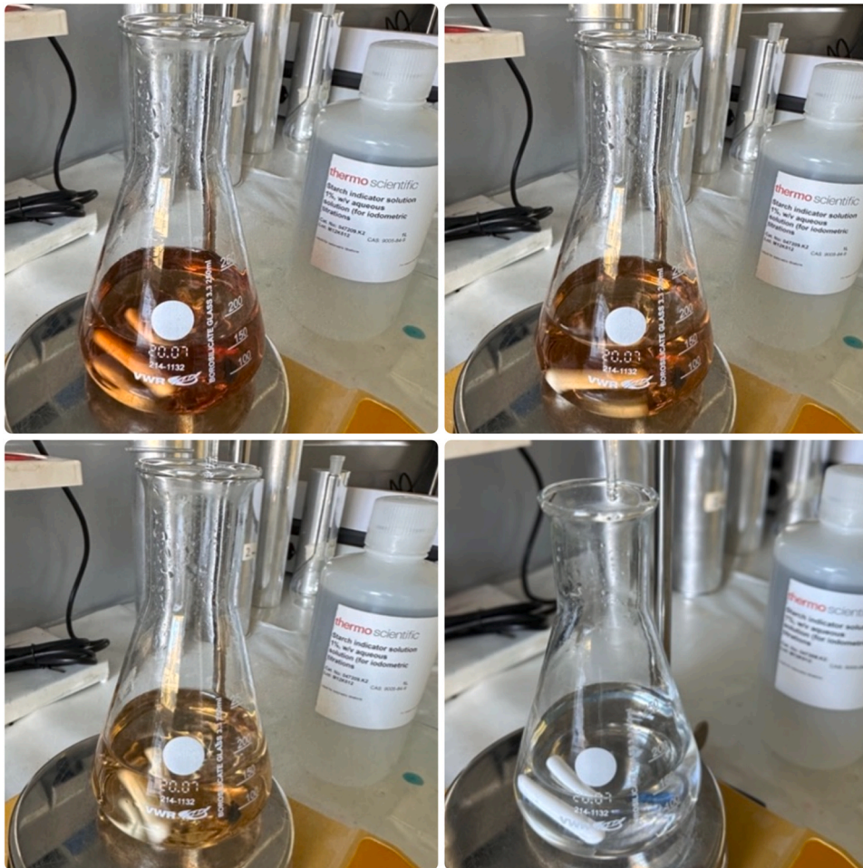
Fig. 1. Pictures of the iodometry procedure. The brownish solution was decoloured with addition of natriumthiosulfate. Starch indicator solution might be added to better recognise the tipping point (see Methods).
