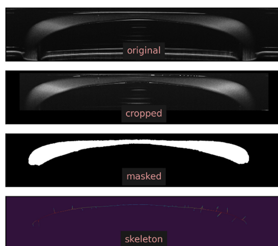
Figure S5. Processing of OCT images in python. The original Tiff-Image is first cropped and bright lines erased. The image is then transferred into a binary mask from which a skeleton is derived.
