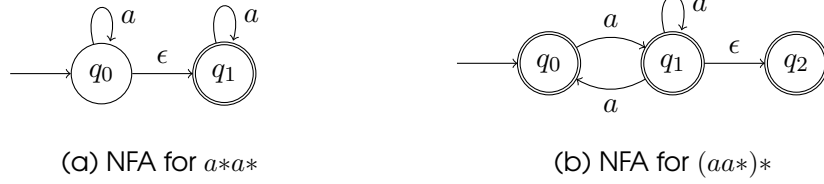
Figure 2.2: Example regexes that, in Spencer’s algorithm, exhibit time complexity that is either: (a) polynomial or (b) exponential; in the length of the input string w = aa...ab .
