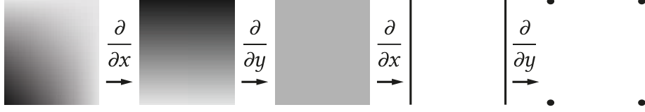
Figure 4.3: Repeated differentiation of a bilinear patch ( d = n = 2 ). After the first differentiation, the patch exhibits linear variation only along the vertical dimension. After subsequent differentiations, we obtain a constant patch, two vertical lines, and, finally, four Dirac deltas.
