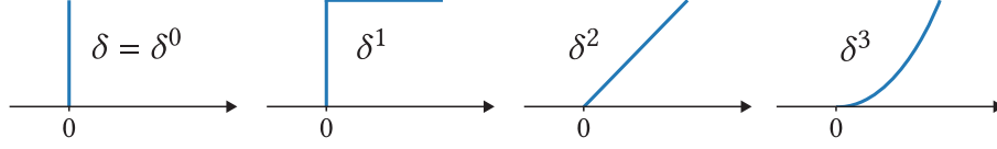
Figure 4.5: 1D ramps of different orders (redrawn from (Heckbert, 1986)). Each ramp is the antiderivative of its predecessor.
