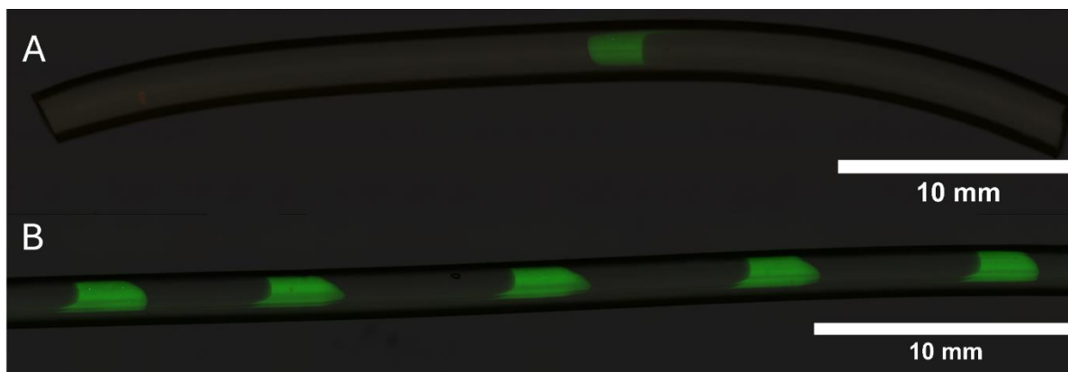
Figure 45. Fluorescent microscopy of the printed core-cladding fiber containing A) single and B) multiple segments of AuNRs ( 0.07 \text{ mg mL}^{-1} ) + Fluospheres. The images are an overlay of the brightfield image, the green fluorescence ( 0.01 \text{ \% w/w} Fluosphere) capturing particle fluorescence.
